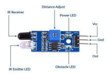
An IR (Infrared) Sensor is an electronic device that detects infrared radiation (heat) emitted by objects or their surroundings. Infrared light is a type of electromagnetic radiation with wavelengths longer than visible light, which makes it invisible to the human eye. IR sensors are commonly used for proximity sensing, object detection, temperature measurement, and communication in a wide range of applications.
