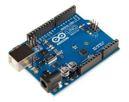
Arduino is an open-source electronics platform that is easy to use for building digital devices and interactive objects. It consists of both hardware (microcontroller boards) and software (Arduino IDE and programming environment), designed to make working with electronics accessible and straightforward, especially for beginners.
